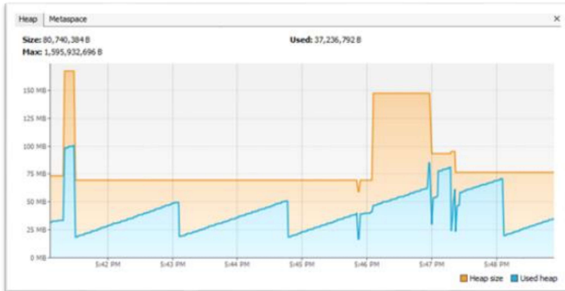
Figure 7 Heap size on the server side can be more turbulent. I think this can be mostly attributed to my use of profiling. The peaks in the graph occurred when I engaged memory profiling. From 5:42 – 5:45 is what could be described as normal operating behavior. Server requests can result in fluctuations in the heap size.
